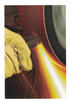
As shown by the sparks in this photo, Cubitron II abrasives divert heat to the swarf, keeping both the workpiece and the belt cooler.
