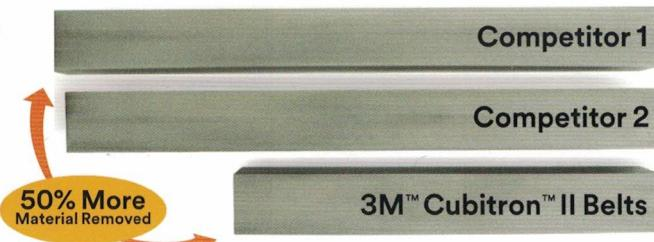
This photo shows three identical 304 stainless steel bars after nine grinding cycles of ten seconds per cycle using equal pressure. In that time, the Cubitron II belt removed more than 50% more metal than the so-called "next-generation" ceramic grain abrasive.
