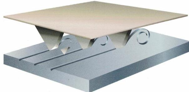
The new precision-shaped grain found in 3M™ Cubitron™ II Belts combines the advanced material properties of our original Cubitron grain with the precise microreplicated structures pioneered in 3M™ Trizact™ Abrasives. As the triangular shaped grain wears, it continuously fractures to form sharp points and edges. The result is a belt that cuts faster, stays cooler and lasts up to 4 times longer than the next best competitive belt.
